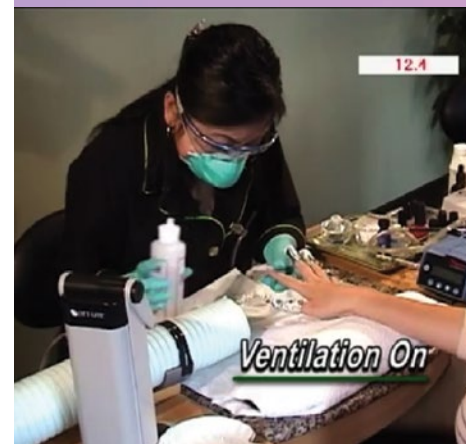
Ventilation on: With a ventilation system running, chemical levels dropped significantly during the same process (below 12.4 parts per million).
